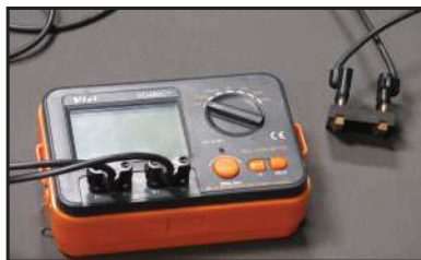
Milli-ohm meter with four point Kelvin probe surface resistivity configuration
