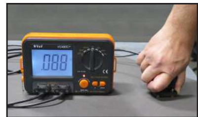
Apply pressure until reading stabilizes. The jig can be rotated in plane to check for directionality
