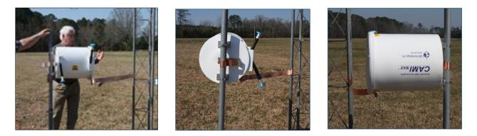
If the **CAMI5000<sup>™</sup>** is attached to a post or ice bridge grounded structure near the tower, "Hot" and "Cold" ends will be reversed!
